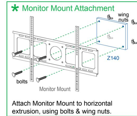
Attach Monitor Mount to horizontal extrusion, using bolts & wing nuts.
