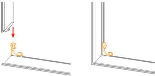
Keep corner connectors attached to horizontal extrusions.
