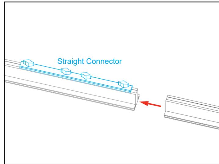
Slide connector across seam of extrusions.
