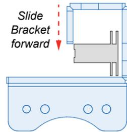
③ Tighten thumb screws to secure connection to inside of frame.
