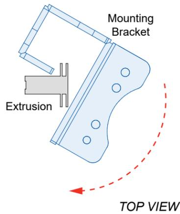
② Slide bracket forward, then down onto V4 connector.
