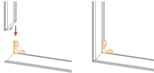
Keep corner connectors attached to horizontal extrusions.
